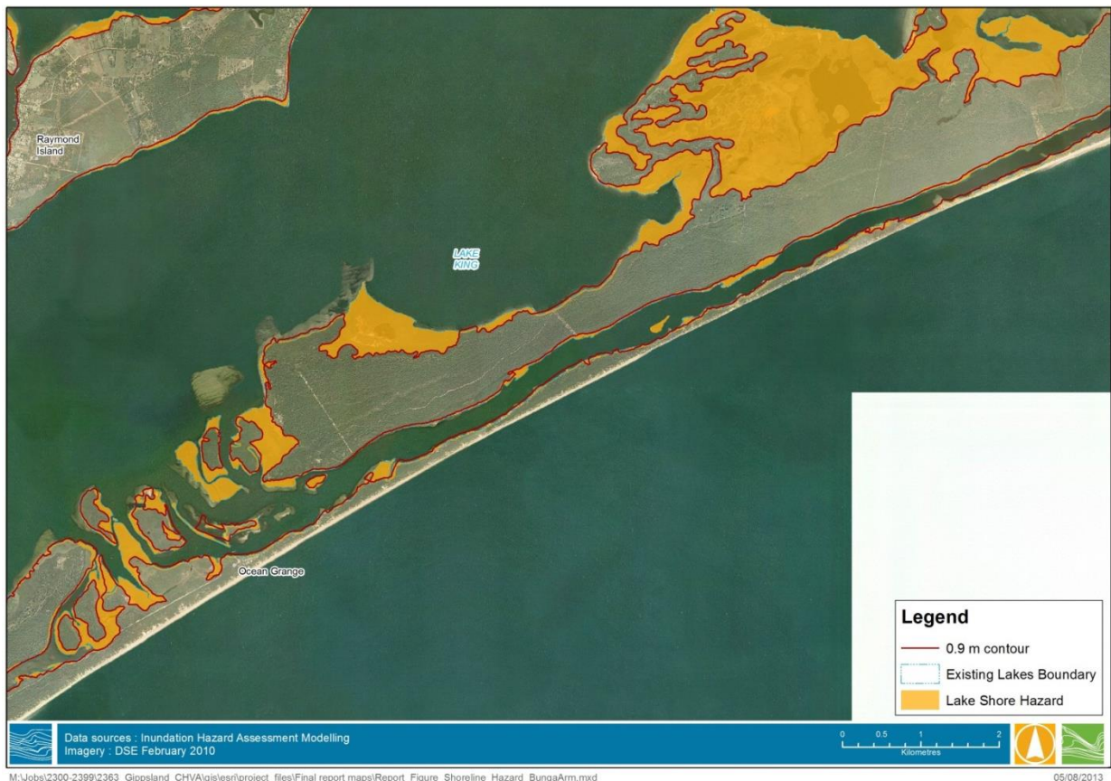
Figure 4-22 Bunga Arm Shoreline Hazard Extent under 0.8 m SLR
