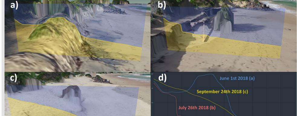
Storm damage before and after a major storm event at Apollo Bay. Red indicates erosion, and blue indicates accretion. a) June 1st 2018, b) July 26th 2018, c) Volumetric comparison between the two dates. Over 430 m3 of sand was lost along a 75 m stretch of beach.
