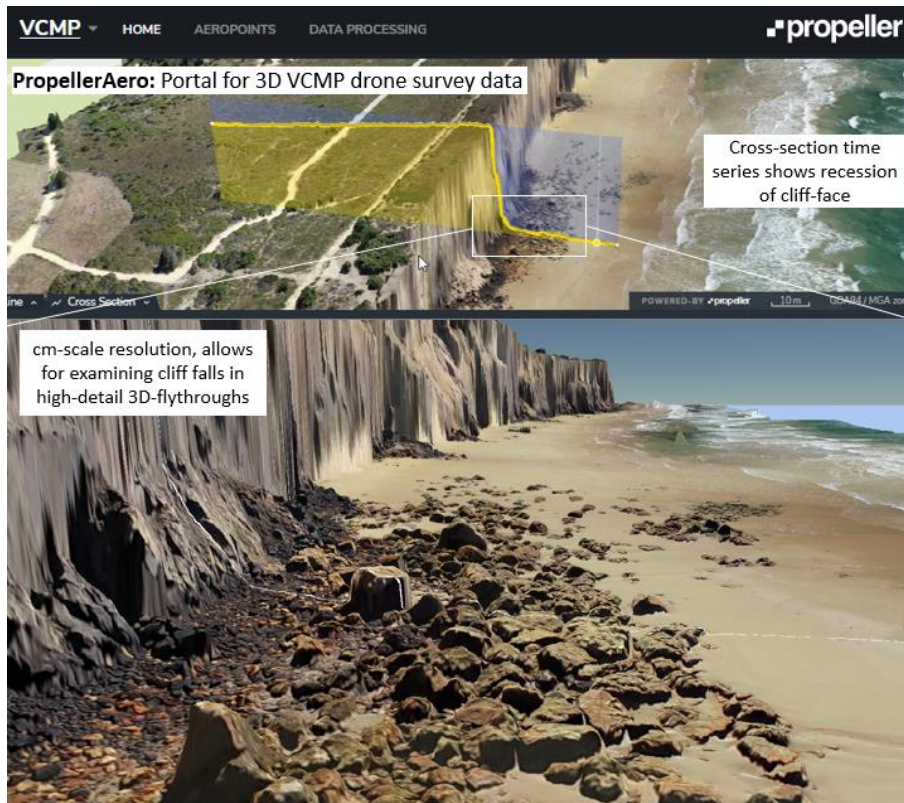
Figure 5. Example analysis from the PropellerAero data processing and hosting portal.
