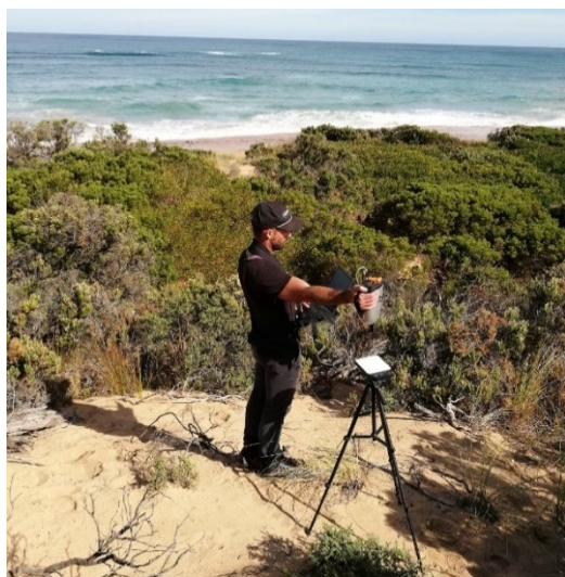
Figure 1: Me, taking hyperspectral signatures of sand from the dune in Warrnambool beach.
