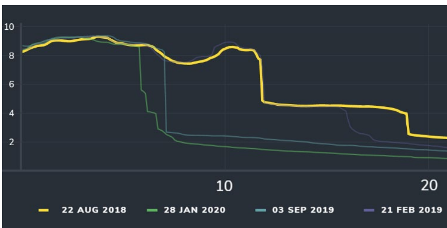
A retreat of 11.6 m was observed at the toe of the dune between August 22, 2018 and January 28, 2020
