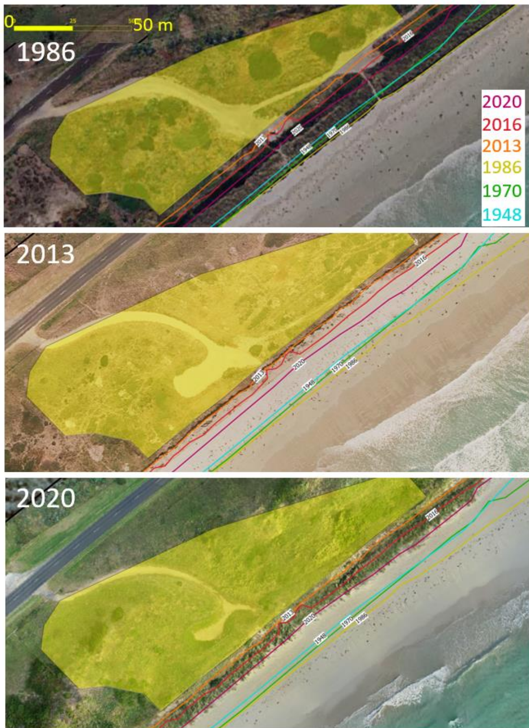
Figure 5-2. Aerial imagery of the DEECA landfill site, overlaid with vegetation line positions. The yellow shaded area is the approx. extent of landfill, based on Tonkin and Taylor (2019).
