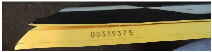
PropellerAero have notified me that this is a manufacturing fault and will be replacing any AeroPoints which start with 003 or 1446 that are delaminating. If you have any of these, could you please email Blake Allan (b.allan@deakin.edu.au) with a photo of the separation, including the number of the AeroPoint (as image above).
