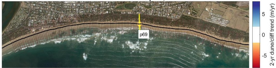
OceanGrove Dune/Cliff Erosion Hotspots, back-level 2.5 m
