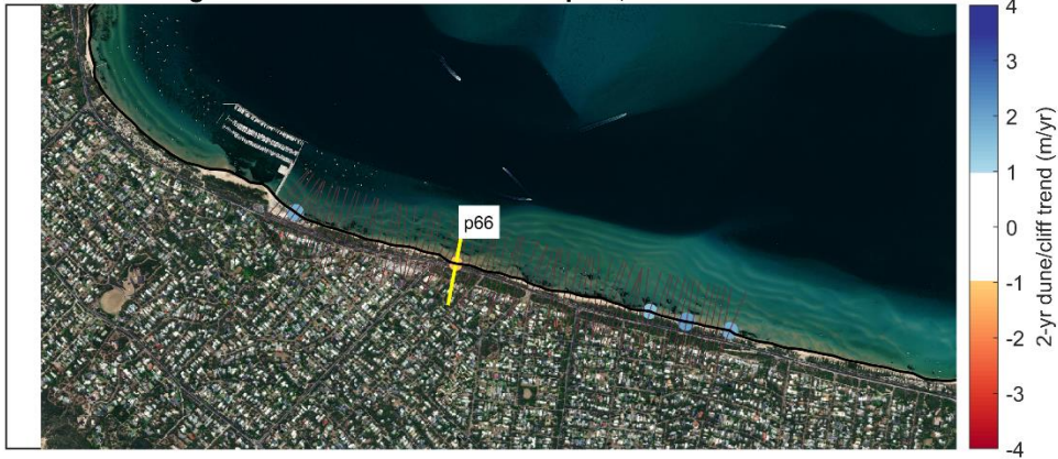
Blairgowrie Dune/Cliff Erosion Hotspots, back-level 1.8 m
