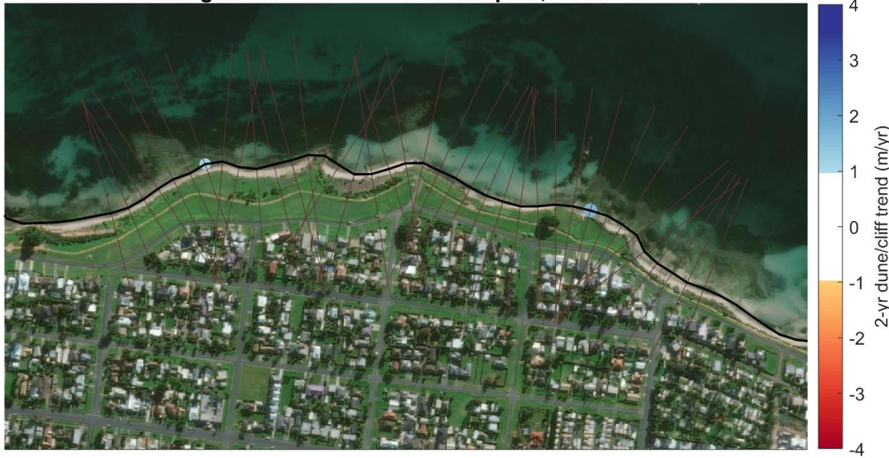
Portarlington Dune/Cliff Erosion Hotspots, back-level 2 m
