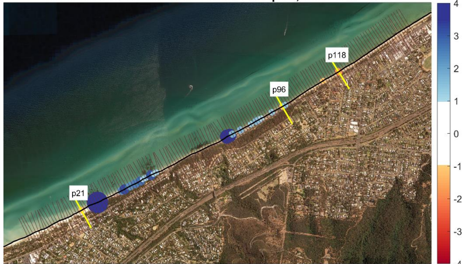
Dromana-McCrae Dune/Cliff Erosion Hotspots, back-level 1.8 m
