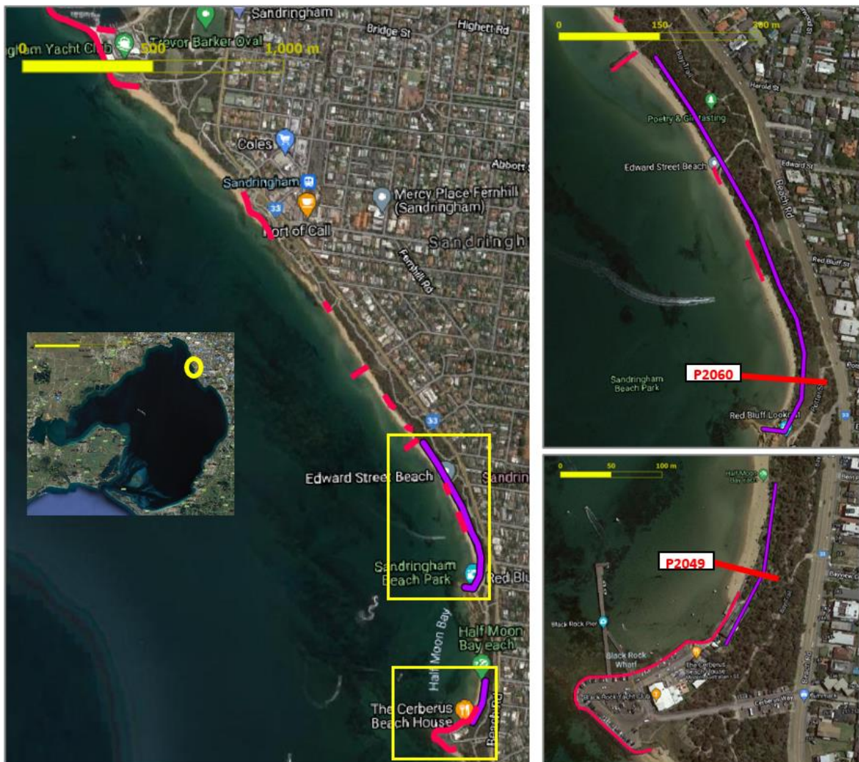
Fig. 3.3.1. Sandringham and Half Moon Bay, drone surveys cover the full extent of left panel. (Top right) South Sandringham nourishment; and (bottom right) Half Moon Bay nourishment. Red lines indicate coastal structures, pink lines are nourishment targets. Two transects indicated in right panels (P2024, P2018) are analysed in detail in Fig. 3.3.6.
