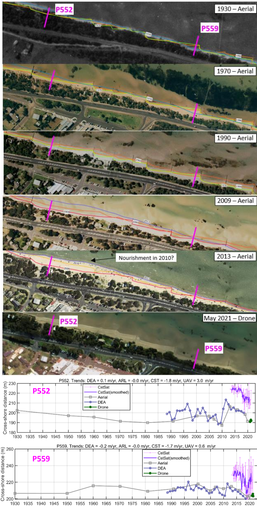
Fig. 3.1.4. Blairgowrie east of Marina nourishment target, (rows 1-5) aerial and drone image time series, (bottom row) multi-method shoreline position time series. Pink line in top panels show location of profile (P552) analysed in bottom panel.
