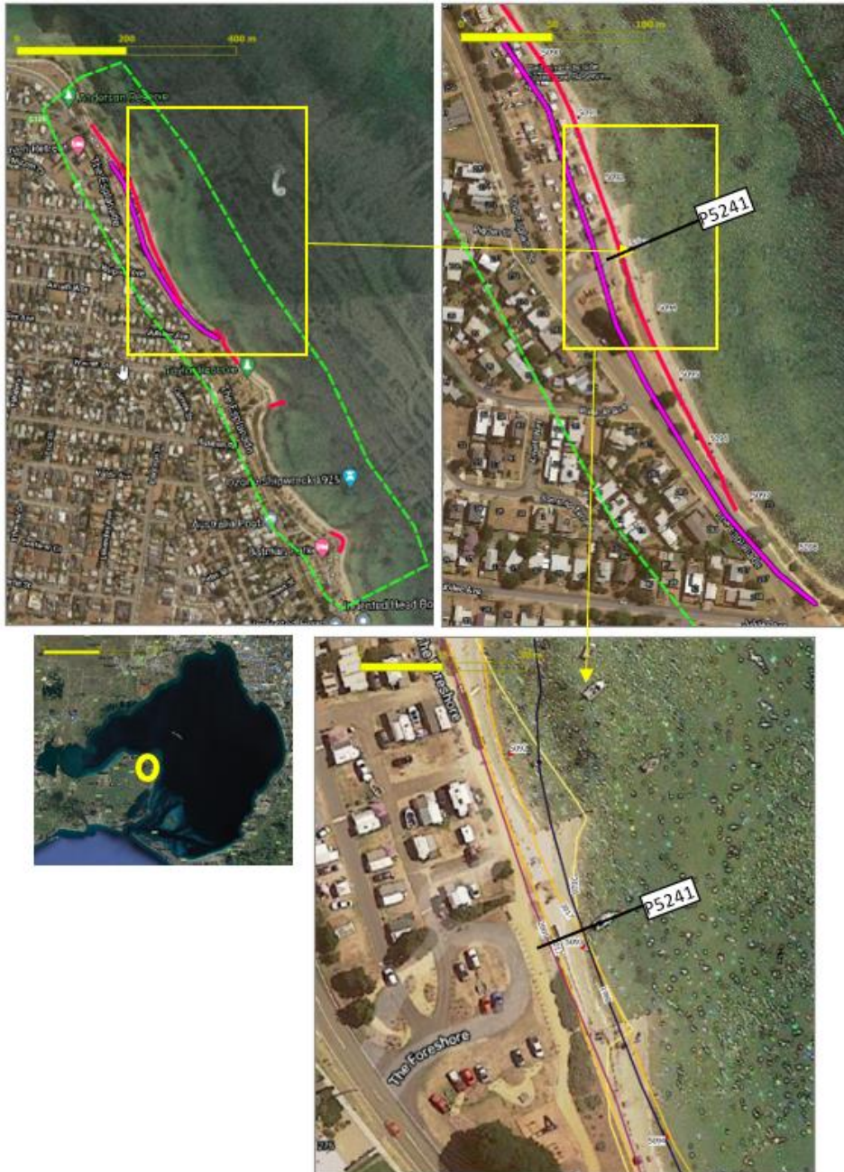
Fig. 3.4.1 Anderson reserve monitoring and nourishment site. Green dashed line is minimum area of drone survey coverage, red lines are coastal structures, pink line is nourishment zone, yellow boxes show progresses levels of zoom.
