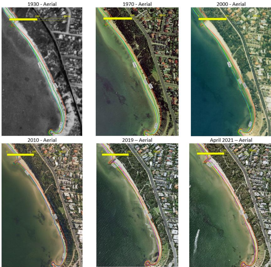
Fig. 3.3.4. Sandringham (south end) aerial photo time series (1930 – 2021).
