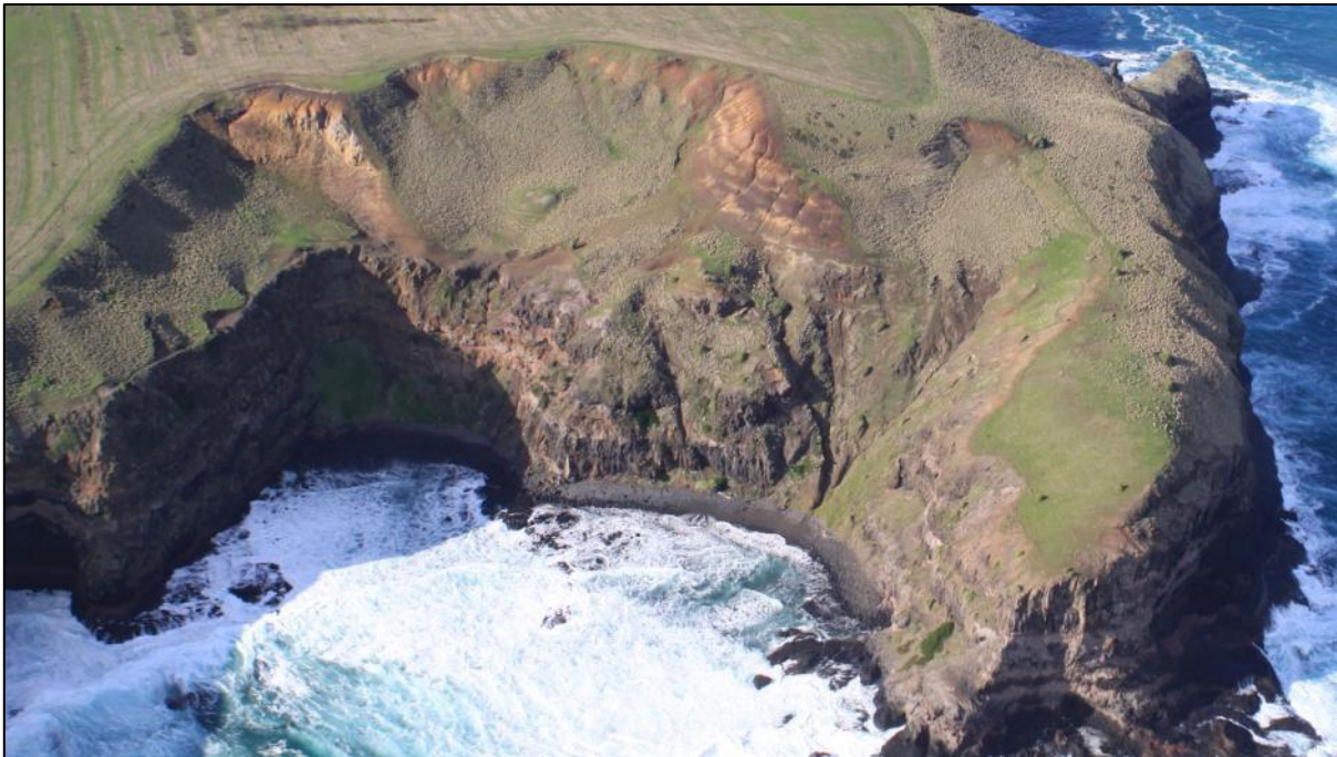
Figure 4-5 Example of Hard Rock Cliff Mass Movement Erosion on the Upper Slopes Including Rotational Sliding Develops a Concave Profile Above a Steep Lower Slope Shaped by Joint Orientation (Source: N Rosengren, 2013)
