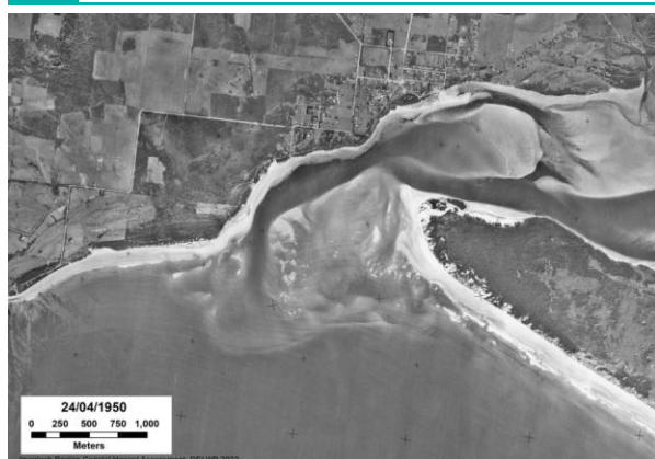
Example historic aerial imagery (1950), used to determine long-term erosion rates. Source: Water Technology
