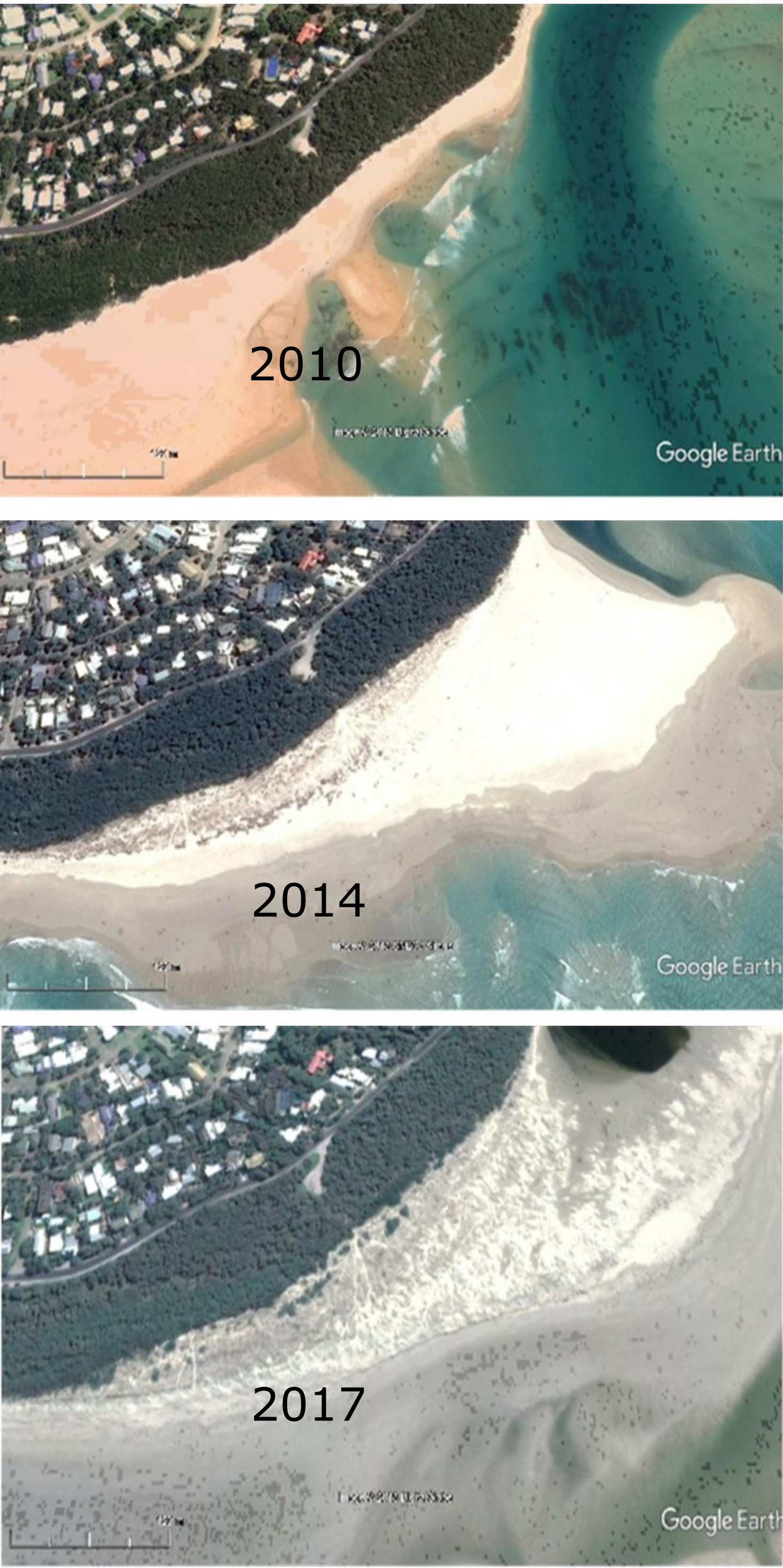
Figure 1: Google earth images of the growth of the sand spit at Inverloch from 2010 to 2017.
