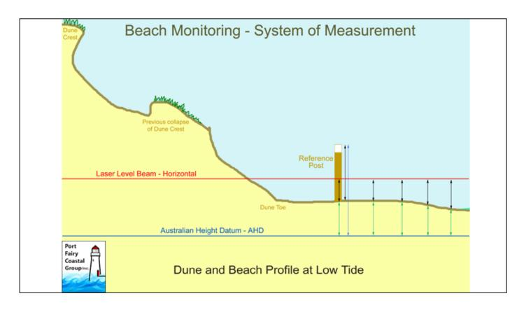
Unlike the dune toe measurements, sand height measurements for beach profile determination involve more readings and the use of a builders laser level to provide a height reference **above** the sand and parallel to the Australian Height Datum.
