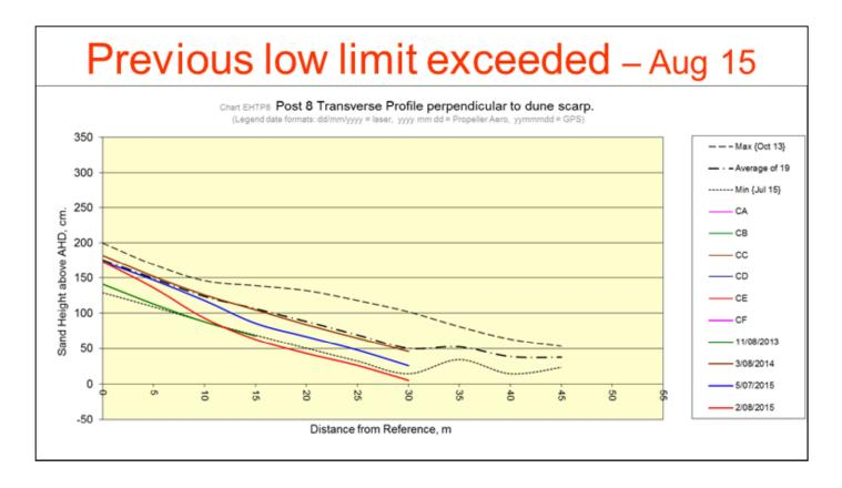
One of the important features developed in earlier spreadsheets was a visual alert to a new low or high value. By setting the statistics date range to be one reading behind the current reading, allows the current profile to plot outside the envelope if its value is greater or less than the previous maximum or minimum at that distance.
