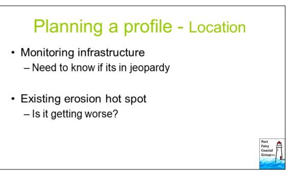
As a general rule, select the part of the beach that is showing the largest erosion and plan a Transverse Profile (Approximately perpendicular to the dune and down to the waters edge) of 30 to 60 metres in length.
