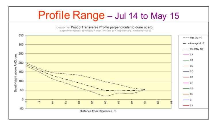
Our discussion on the previous page was prior to the installation of the WEDs rock wall. This chart shows the envelope of profiles in the year following the installation of the WEDs rock wall.
