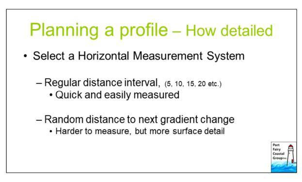
There are two main options for locating the horizontal distance of the point where the vertical height to the laser beam is measured:
