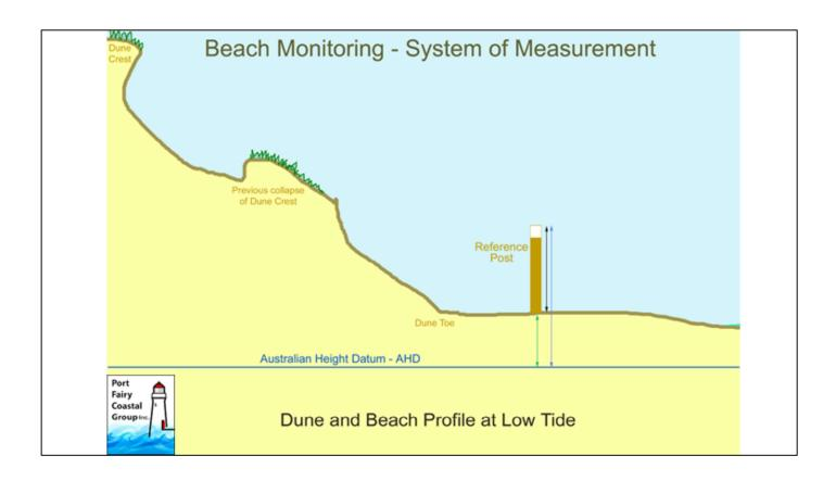
If the post height above the datum is known and the length of post above the sand measured, the sand height above the datum can be calculated. This sand height can then be compared to other parts along the beach.
