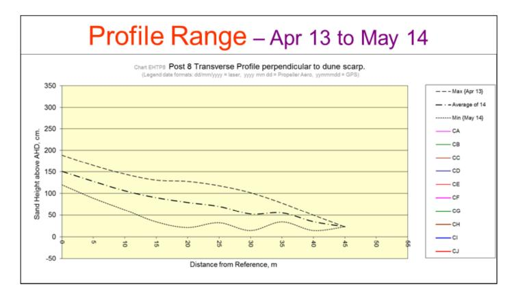
Now that we understand the Max, Min and Average lines, we can set specific ranges of dates and study the effects of any changes in the profiles before and after modifications on the beach.
