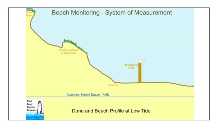
To fully understand beach profiling, we need to define what we will measure and where the measurements will be made.
