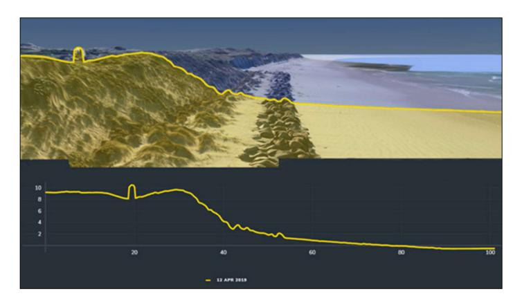
A beach profile is a cross sectional view of the beach to show how the height of the sand changes as you move over the beach. Vertical heights are measured relative to the Australian Height Datum
