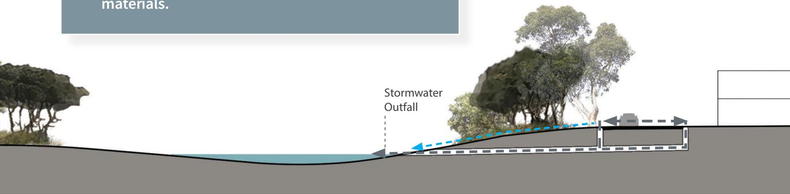
Replace traditional stormwater outfalls with wetlands and biofiltration systems to enhance vegetation and habitat, and ensure environmentally-responsible discharge of water
