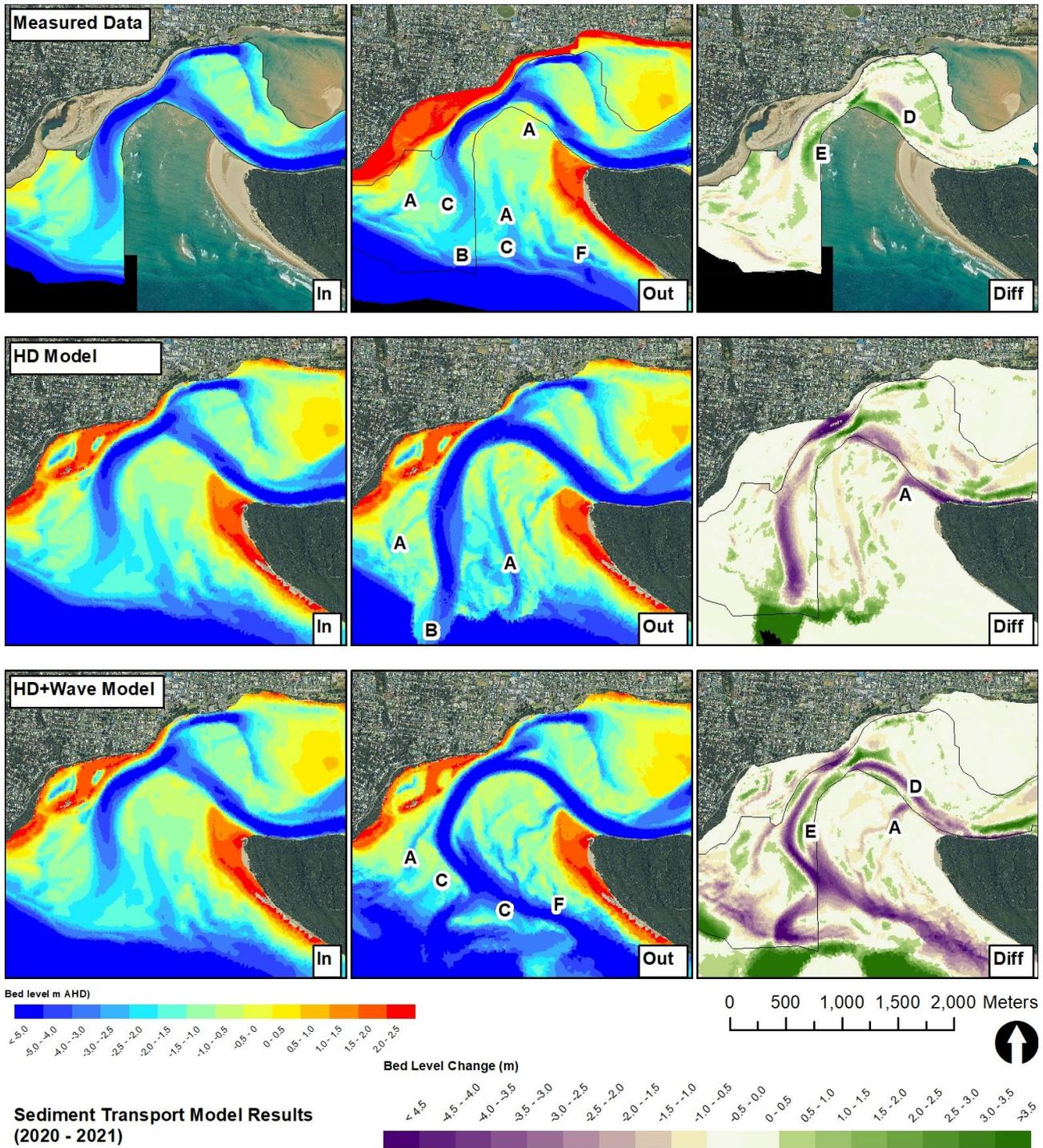
**FIGURE E-17 SEDIMENT TRANSPORT MODEL RESULTS**
