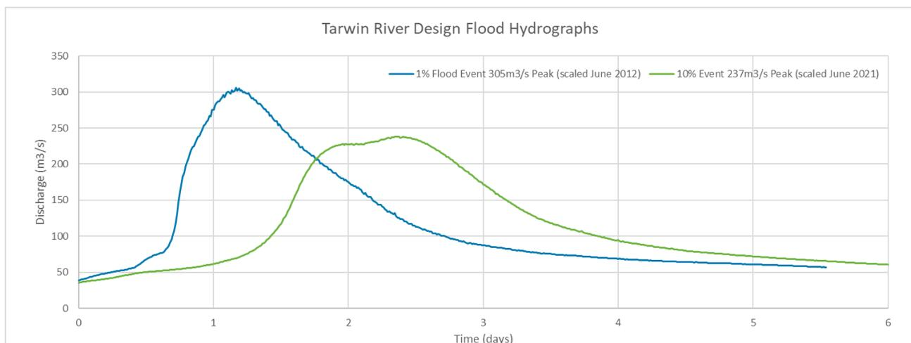
**Figure 3-2 Design Flood Hydrographs**
