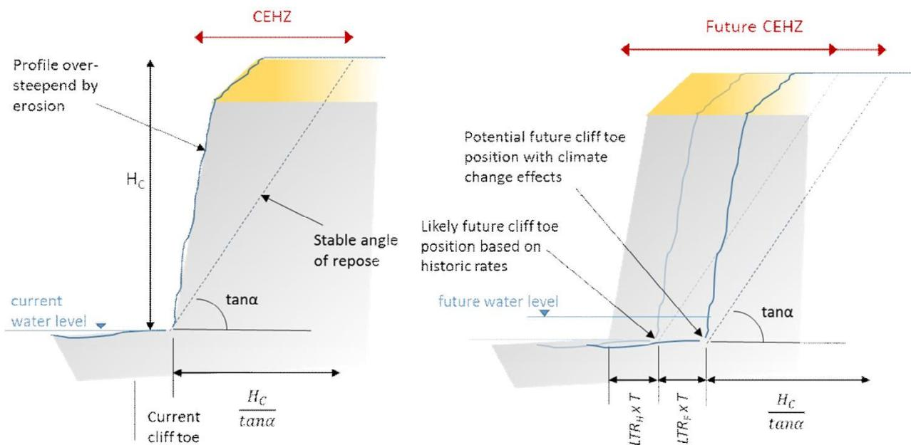
FIGURE F-3 LONGTERM RESSION OF CLIFFED SHORLINES (SHAND ET AL, 2015)
