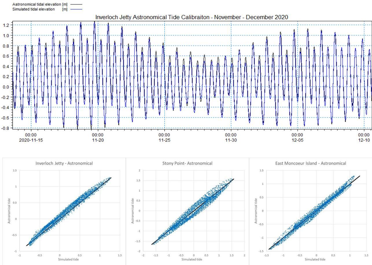
**FIGURE E-5 OCEAN MODEL ASTRONOMICAL TIDE CALIBRATION**
