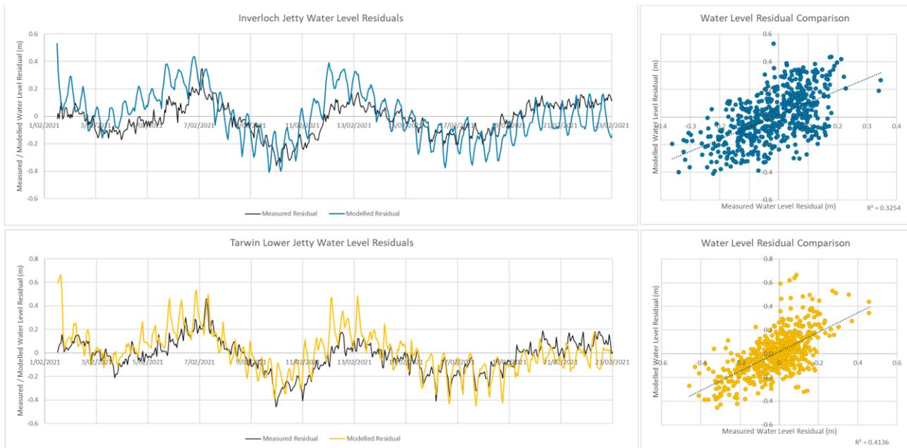
**FIGURE E-12 MODELLED VERSUS MEASURED WATER LEVEL RESIDUALS – CALIBRATION FEBRUARY 2021**
