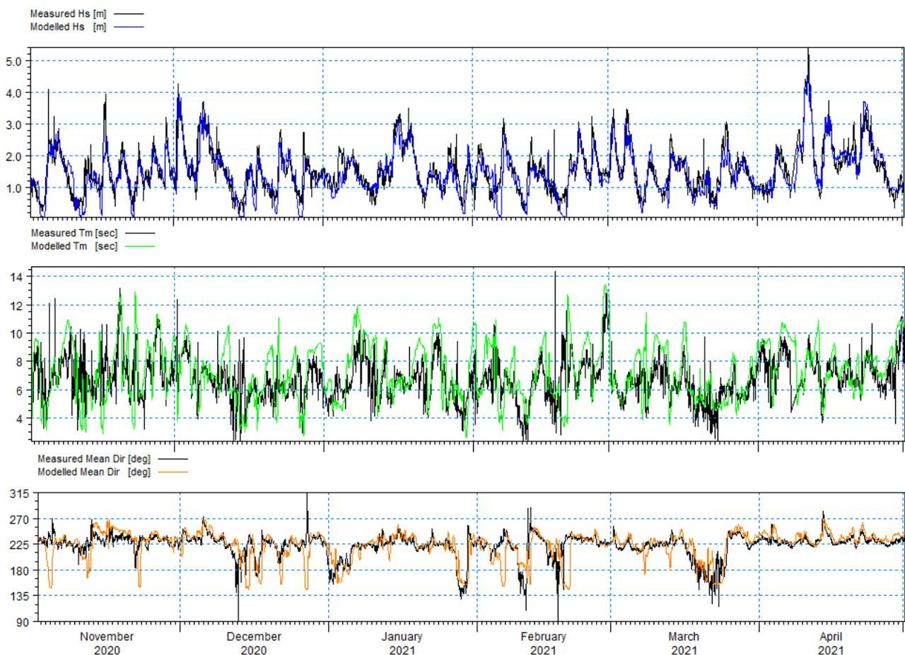
**FIGURE E-7 VERIFICATION OF COUPLED WAVE AND HYDRODYNAMIC OCEAN MODEL WITH MEASURED WAVE DATA**
