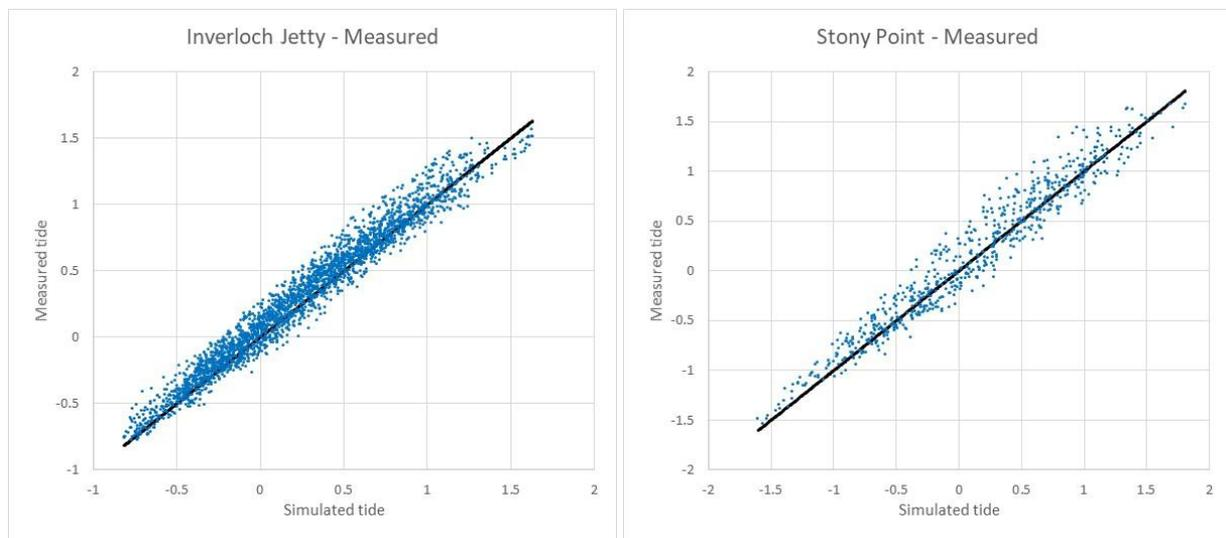
**FIGURE E-6 OCEAN MODEL MEASURED WATER LEVEL VALIDATION**
