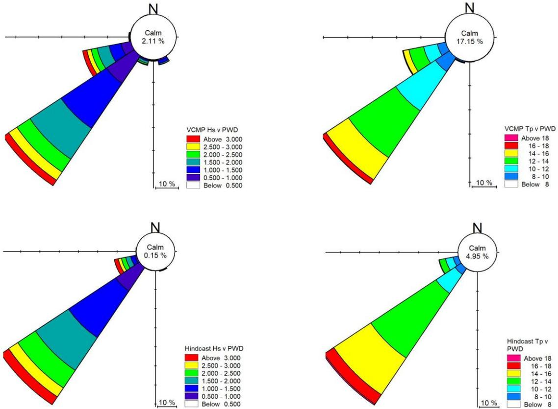
**FIGURE C-2 VCMP OBSERVED (TOP) VERSUS UNIVERSITY OF MELBOURNE HINDCAST (BOTTOM) SIGNIFICANT WAVE HEIGHT (LEFT) AND PEAK WAVE PERIOD (RIGHT) IN VENUS BAY**
