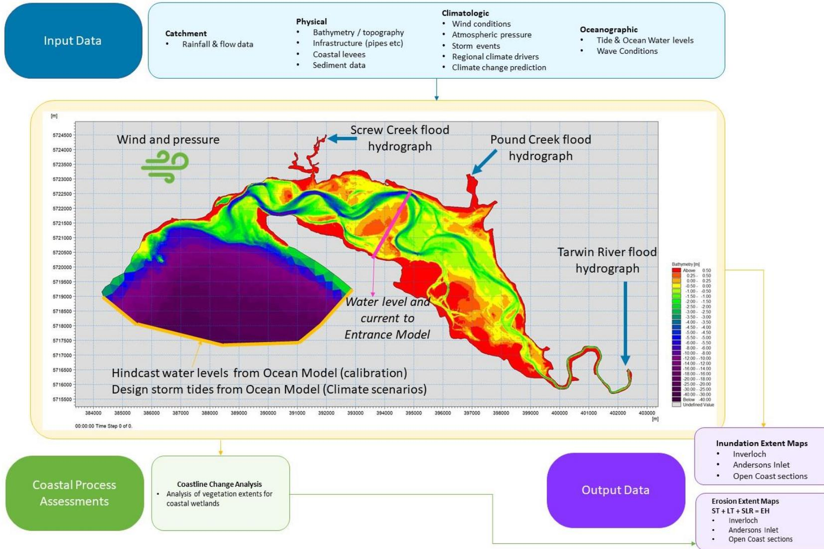
FIGURE E-8 ANDERSON INLET MODEL INPUTS/OUTPUTS
