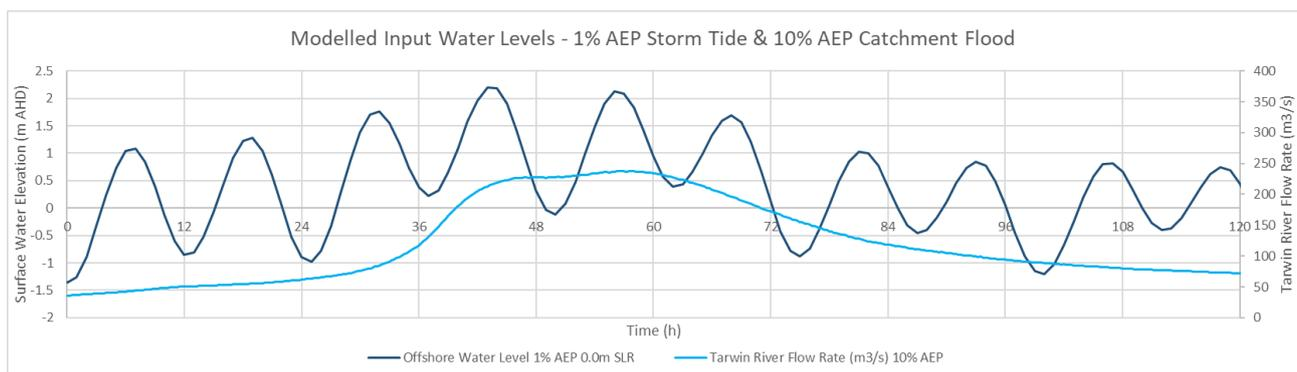
**Figure E-10 Synthesised Storm Tide Boundaries and Flood Events**
