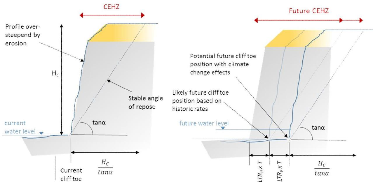
**FIGURE 4-3 LONGTERM RESSION OF CLIFFED SHORELINES (SHAND ET AL 2015)**
