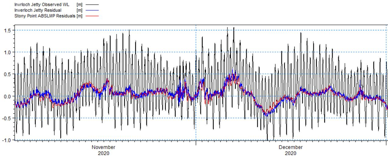
**FIGURE E-4 TIDAL RESIDUALS MEASURED AT INVERLOCH JETTY AND STONY POINT**
