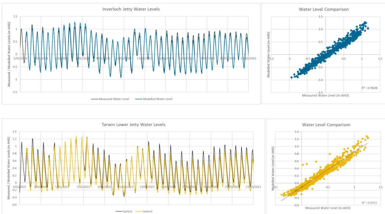
**FIGURE E-11 MODELLED VERSUS MEASURED WATER LEVELS – CALIBRATION FEBRUARY 2021**
