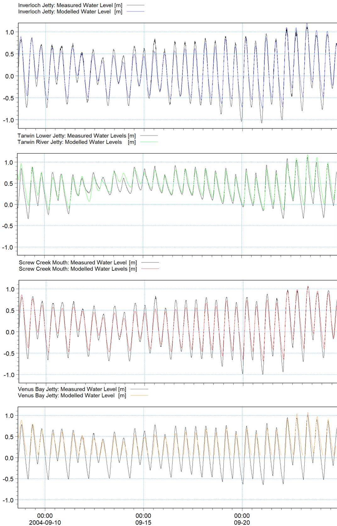
**FIGURE E-14 MODELLED VERSUS MEASURED WATER LEVELS – SEPTEMBER 2004**
