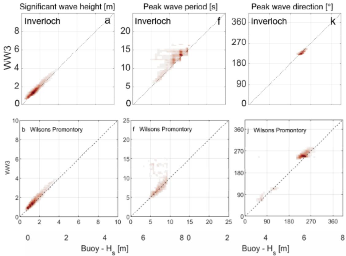
FIGURE C-1 COMPARISON OF MEASURED AND MODELLED WAVES, LIU 2021
