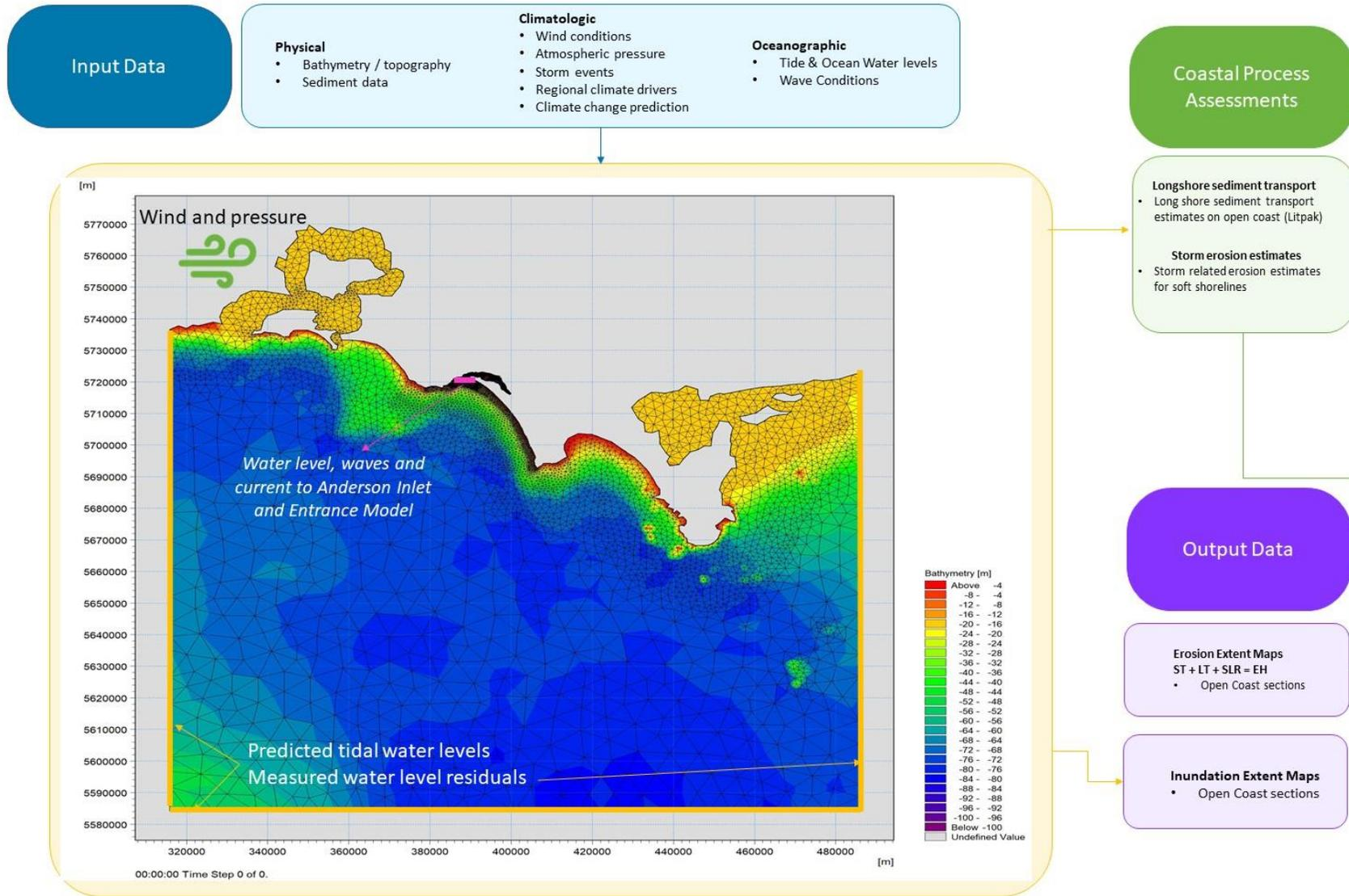
FIGURE E-2 OCEAN HYDRODYNAMIC MODEL INPUTS/OUTPUTS
