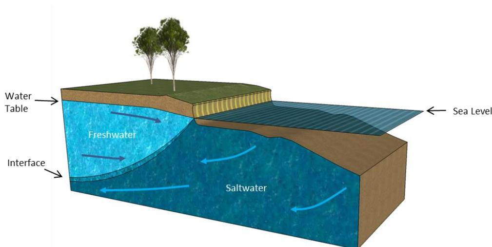
**Figure 4-1** Conceptual freshwater-saltwater interface in an unconfined coastal aquifer
