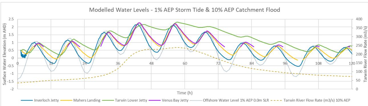
**Figure 3-8 Timeseries of water surface elevation, Anderson Inlet, Existing 1% AEP Storm Tide, 1% Wind + 10% catchment flood**
