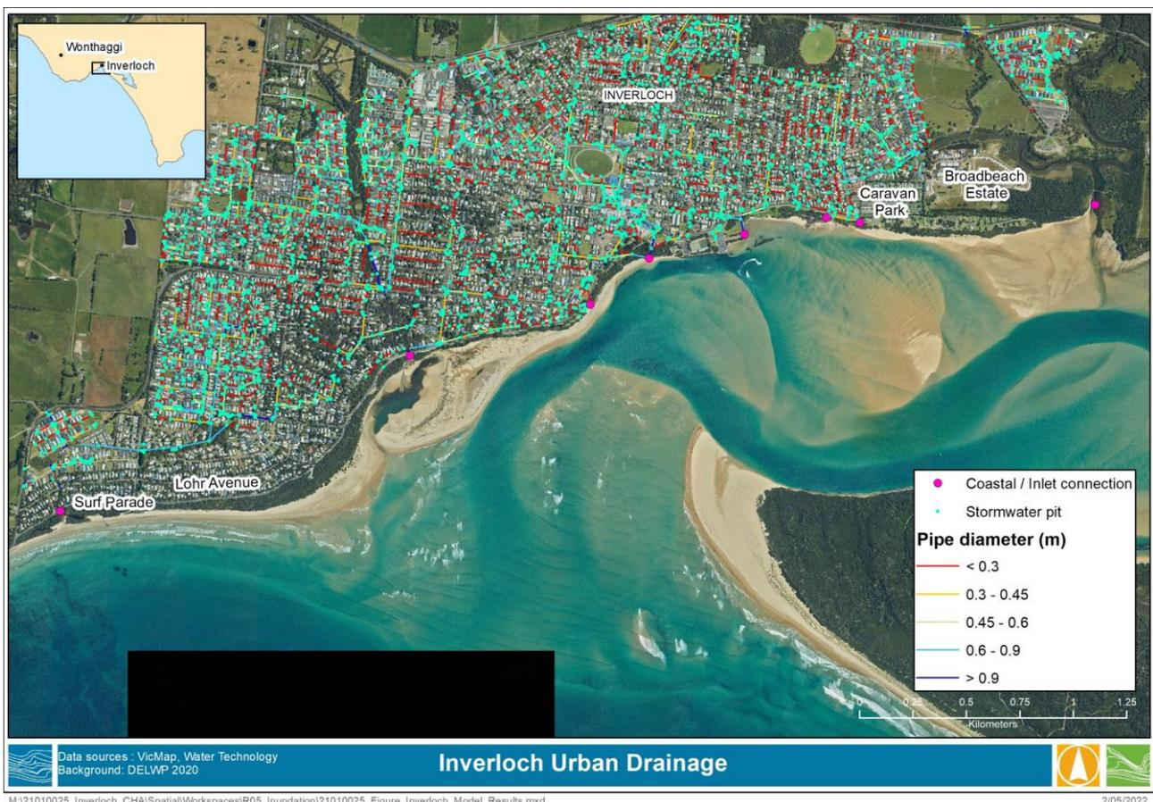
**Figure 2-8 Inverloch Modelled Stormwater Drainage Network**
