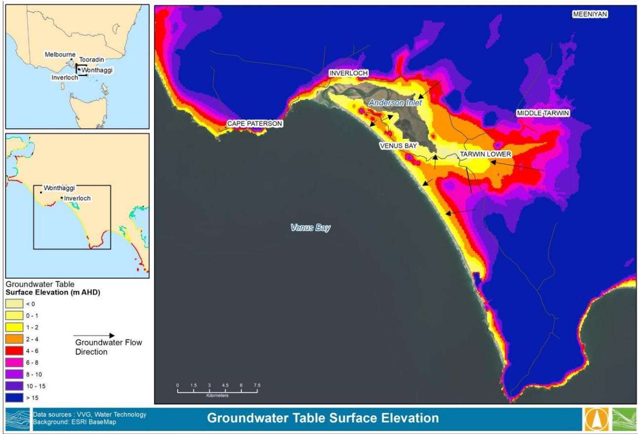
**Figure 4-9 Groundwater Table Surface Elevation and Flow Direction**
