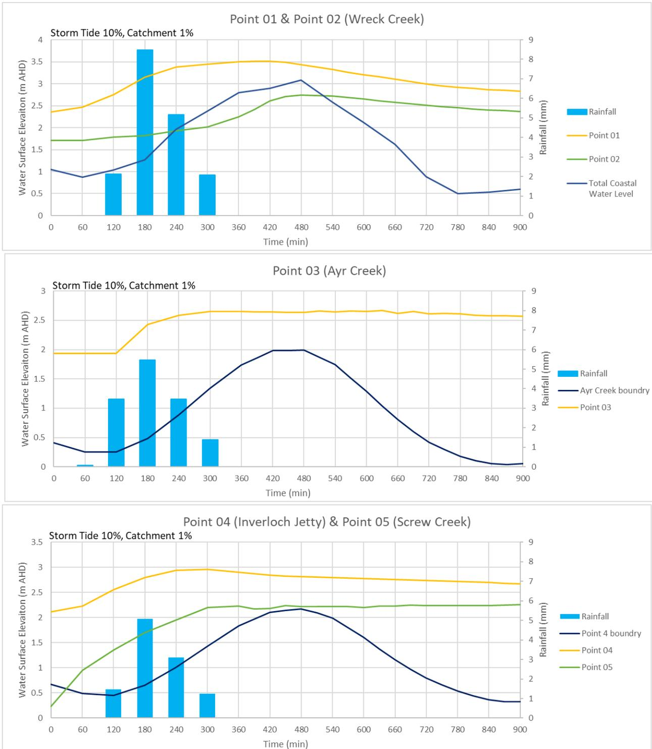
**Figure 3-13 Time varying water levels, Existing 10% AEP Storm Tide + 1% Inverloch Catchment**
