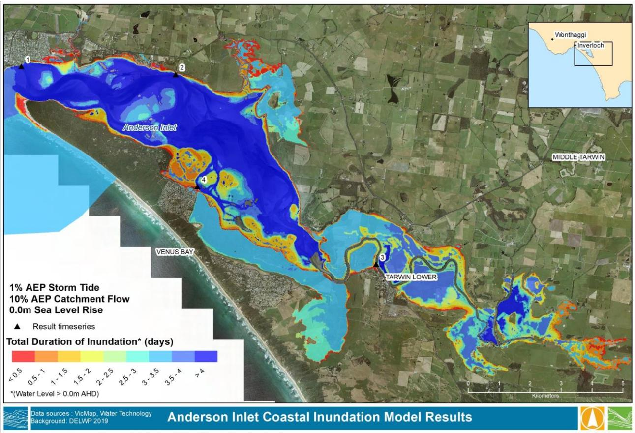
**Figure 3-7 Duration of inundation, Anderson Inlet, Existing 1% AEP Storm Tide, 1% Wind + 10% catchment flood**
