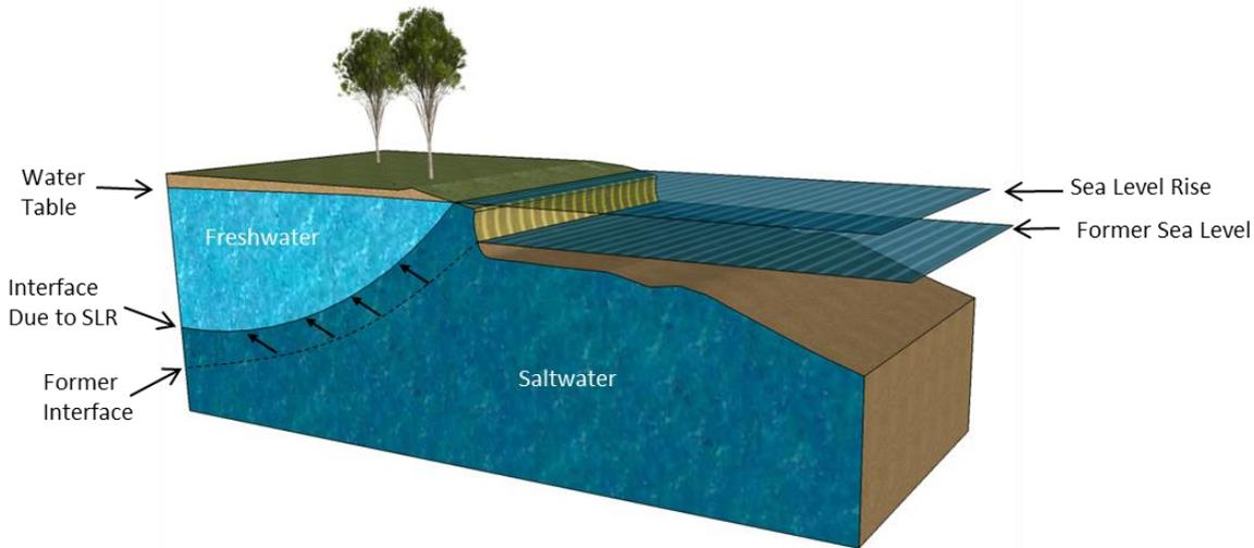
Figure 4-2 Upward and Landward shift in the Freshwater-Saltwater Interface as a result of SLR
