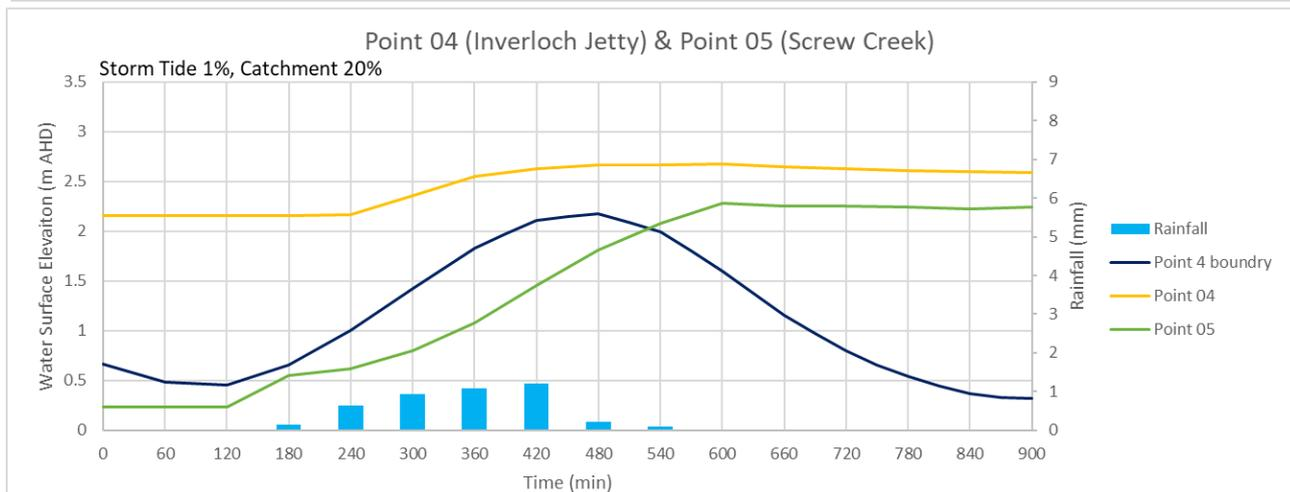
**Figure 3-14 Time varying water levels, Existing 1% AEP Storm Tide + 20% Inverloch Catchment**
