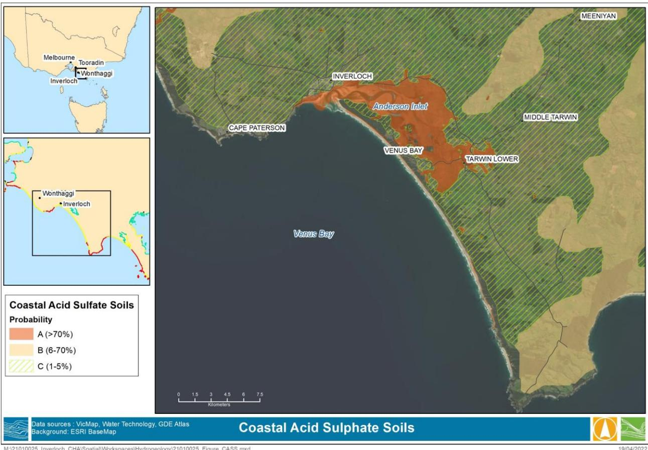
Figure 4-12 Areas of Potential Coastal Acid Sulphate Soil
