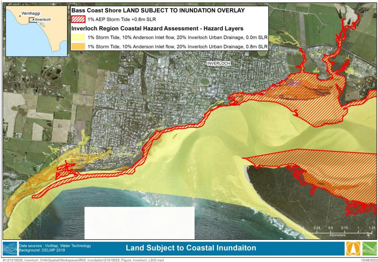
Figure 3-15 Bass Coast LSIO at Inverloch compared with Coastal Inundation Hazard Zones
