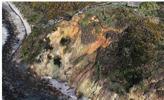
Example of a section of the cliff reconstruction highlighting the erosion near stairs at Portland (3D photogrammetry extract).
