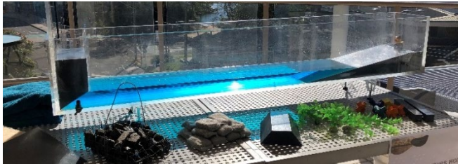
Picture 2: A wave tank is a simple physical model (DEECA)
