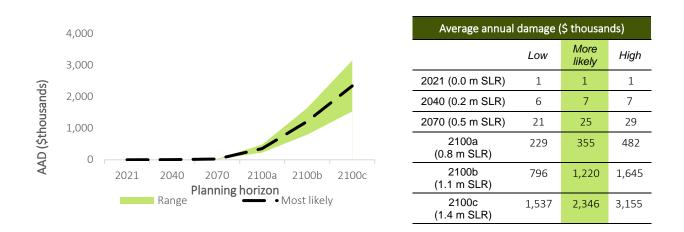
Figure 24. Estimated average annual damage to buildings and facilities – permanent inundation
