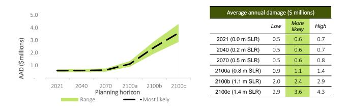
Figure 26. Estimated average annual damage to buildings and facilities – temporary inundation
