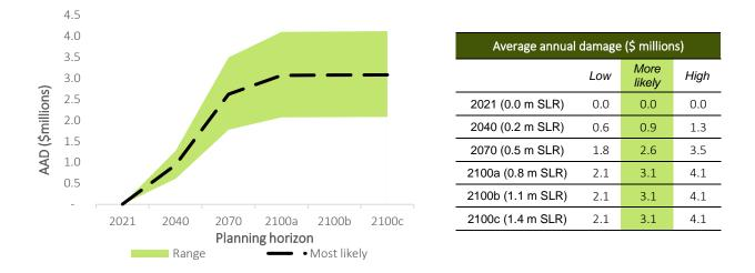
Figure 28. Estimated average annual damage to other infrastructure and utilities – rapid rate erosion scenario
