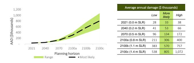
Figure 32. Estimated average annual damage to transport infrastructure – permanent inundation
