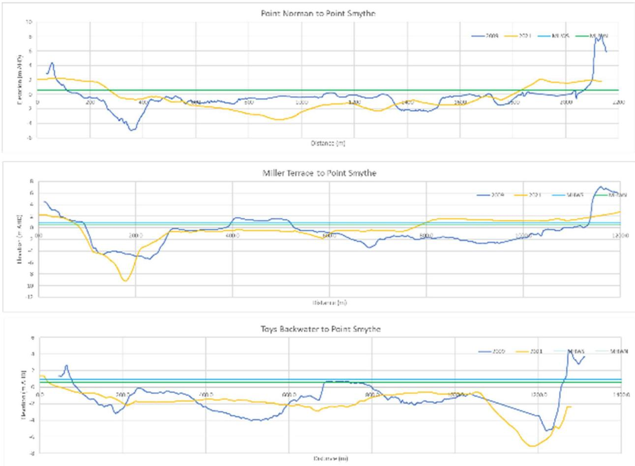
Figure 2-29 Entrance Cross Sections (looking upstream), 2009 v 2021
