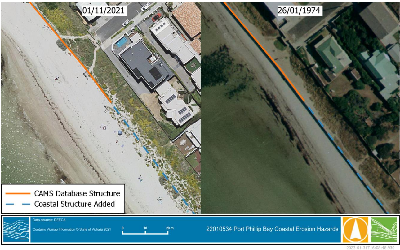
Figure 2-7 Example of area with no structure in the CAMS database but clearly a seawall visible
