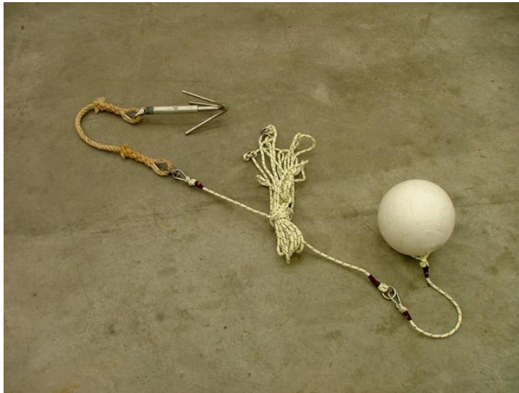
Grapple with Throwline: Note end-of-line float and biodegradable trace behind grapple
