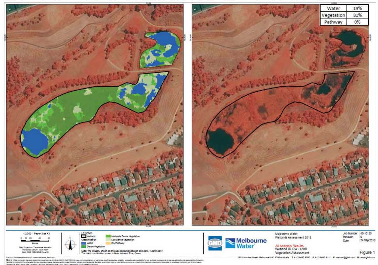
Figure 7: Melbourne Water's satellite IR (infrared) imagery to detect wetland vegetation cover
