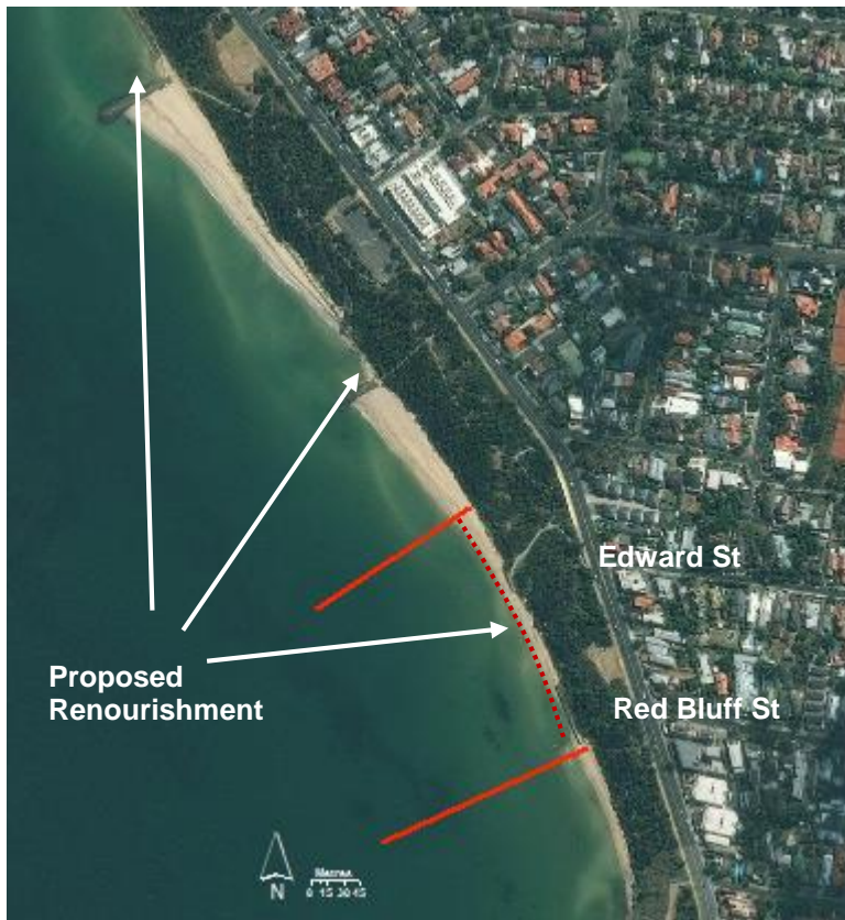
Figure 5-3 Beach renourishment locations including potential alignment of new beach between Profile 2 and 3 (dotted line).
