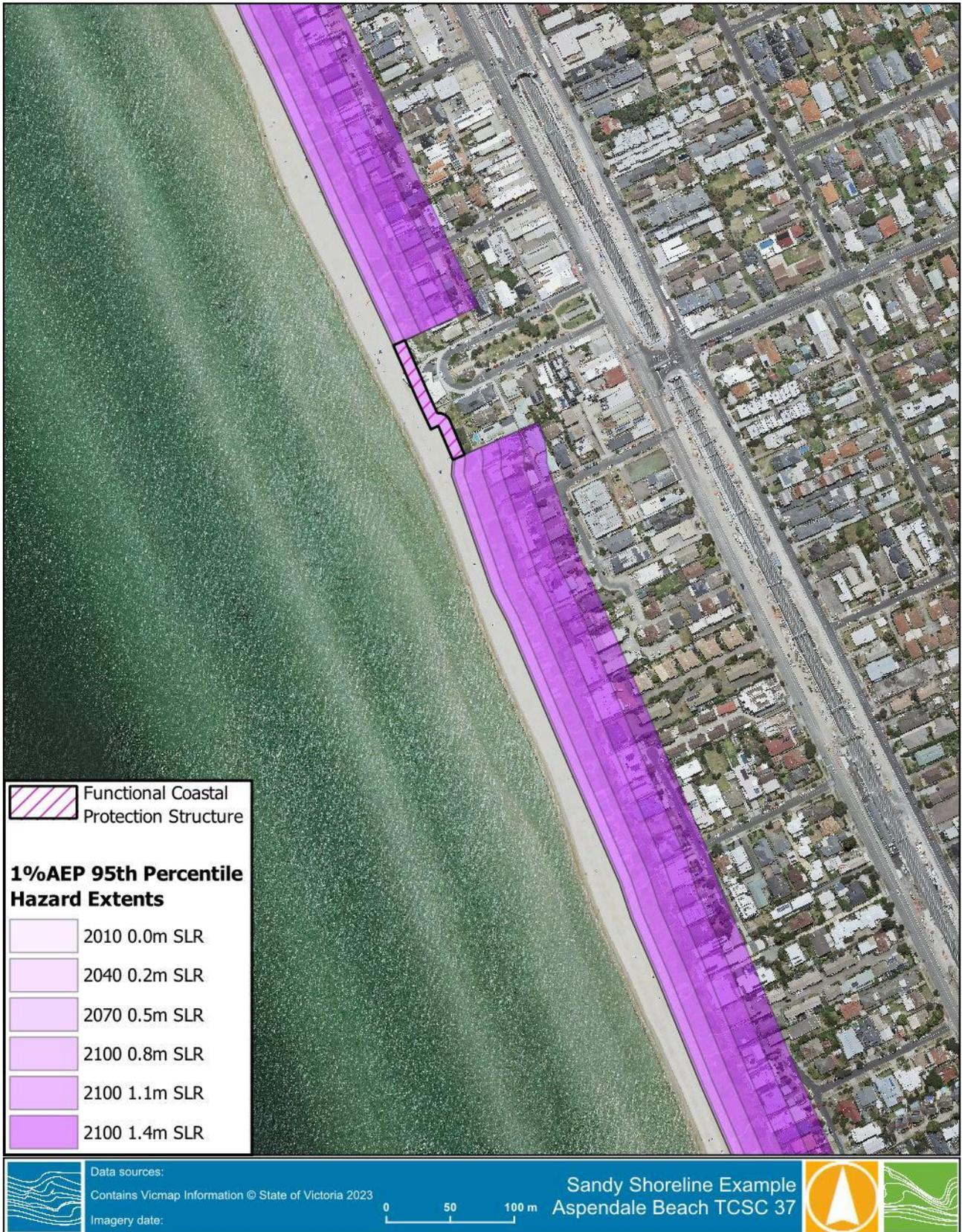
Figure 5-6 Sandy Shoreline Example from 95<sup>th</sup> Percentile 1% AEP
