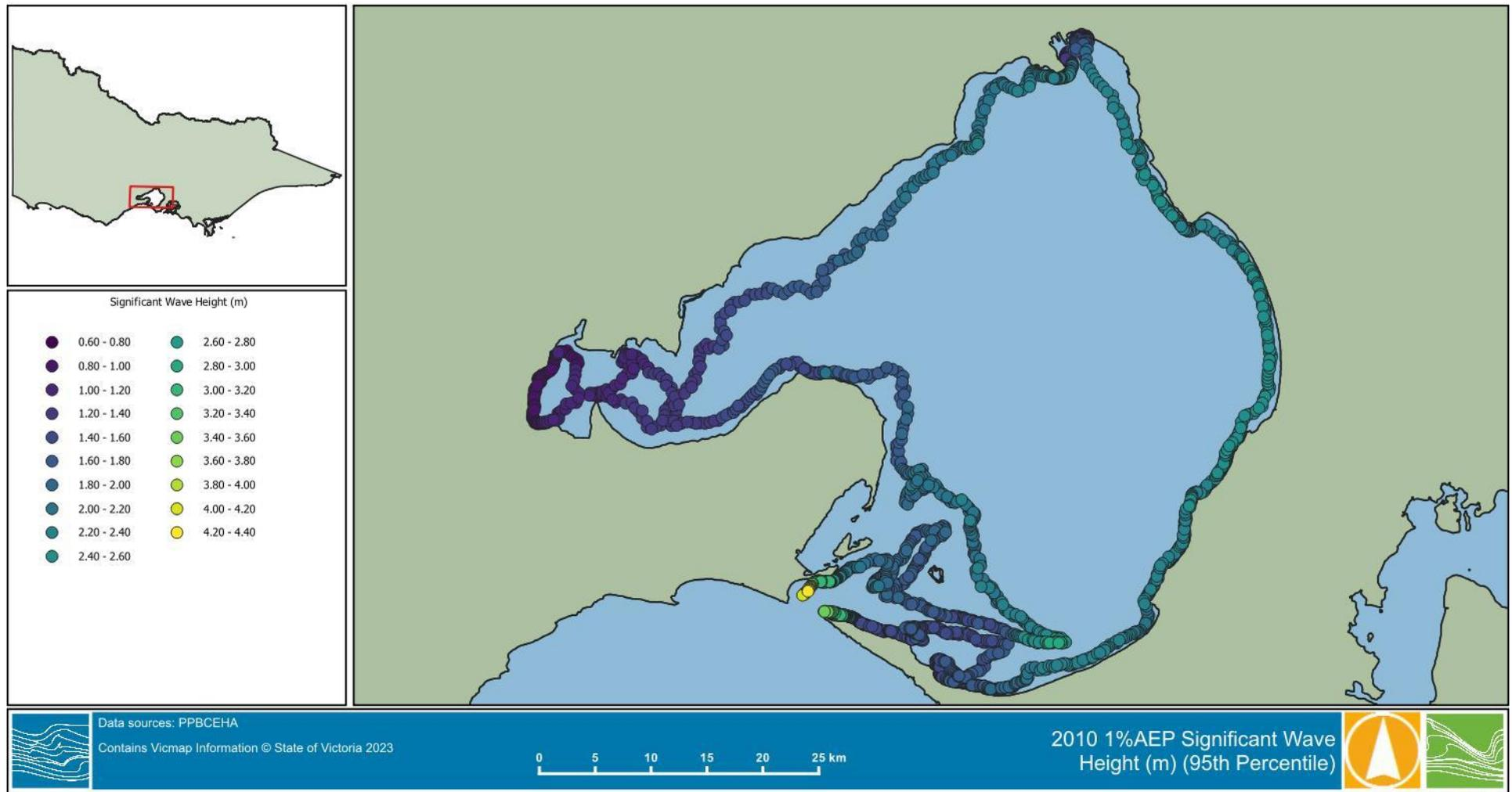
Figure 2-4 PPBCHA 1% AEP Wave Heights
