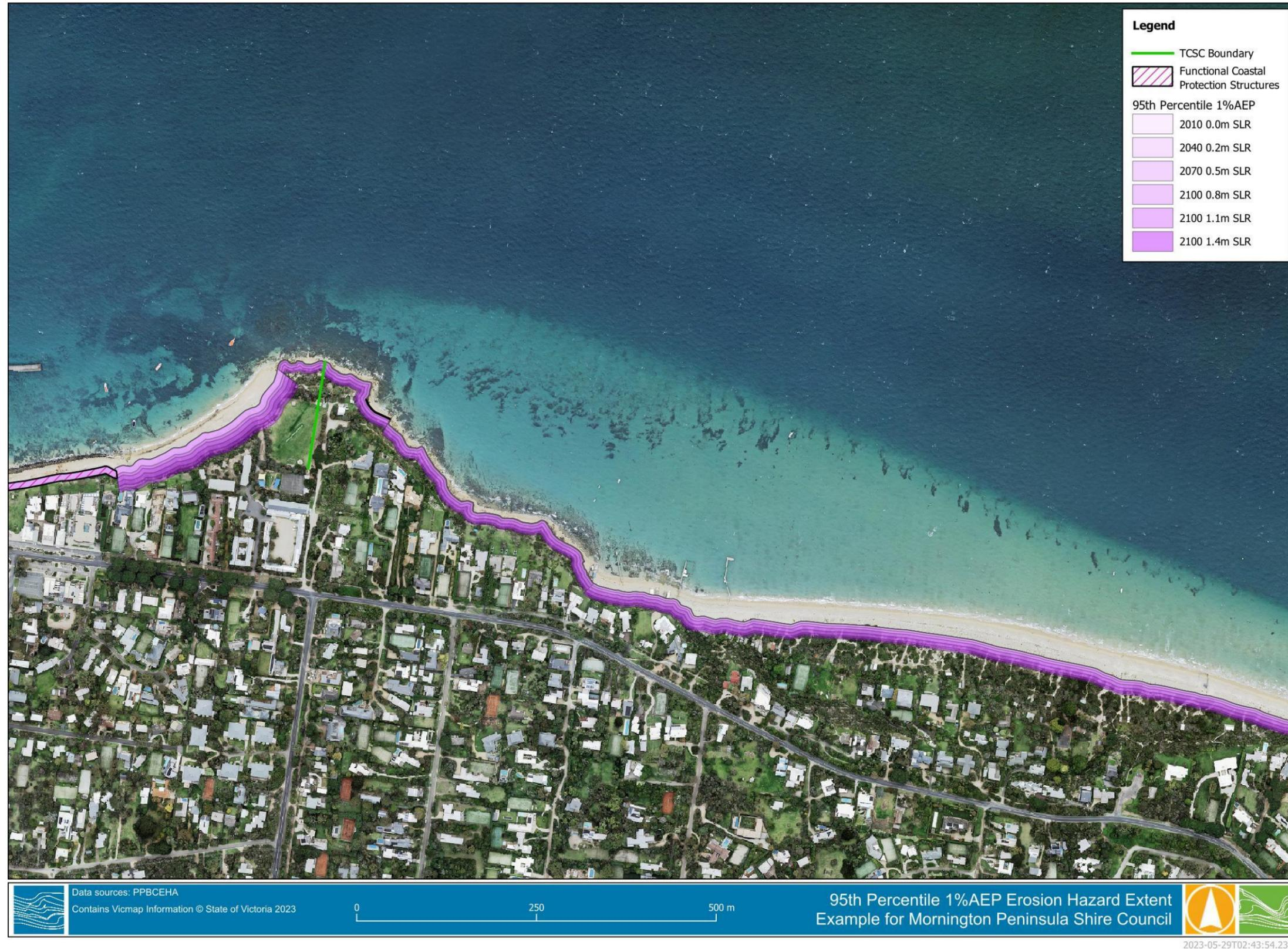
Figure 5-10 95<sup>th</sup> Percentile 1% AEP Erosion Hazard Extent Example for Mornington Peninsula Shire Council
