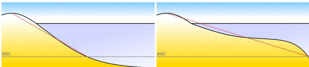
Figure 3-15 Depiction of Bruun Slopes for a classic concave up profile (Left); and a convex profile (Right)
