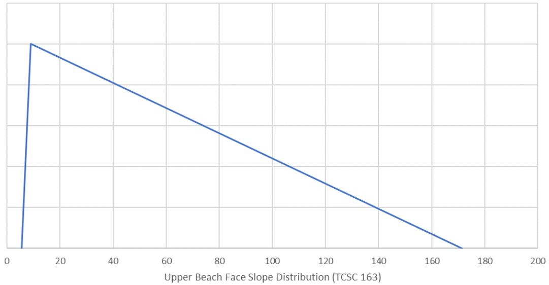
**Figure 3-17 Triangular Distribution of upper beach face slope (TCSC 163)**
