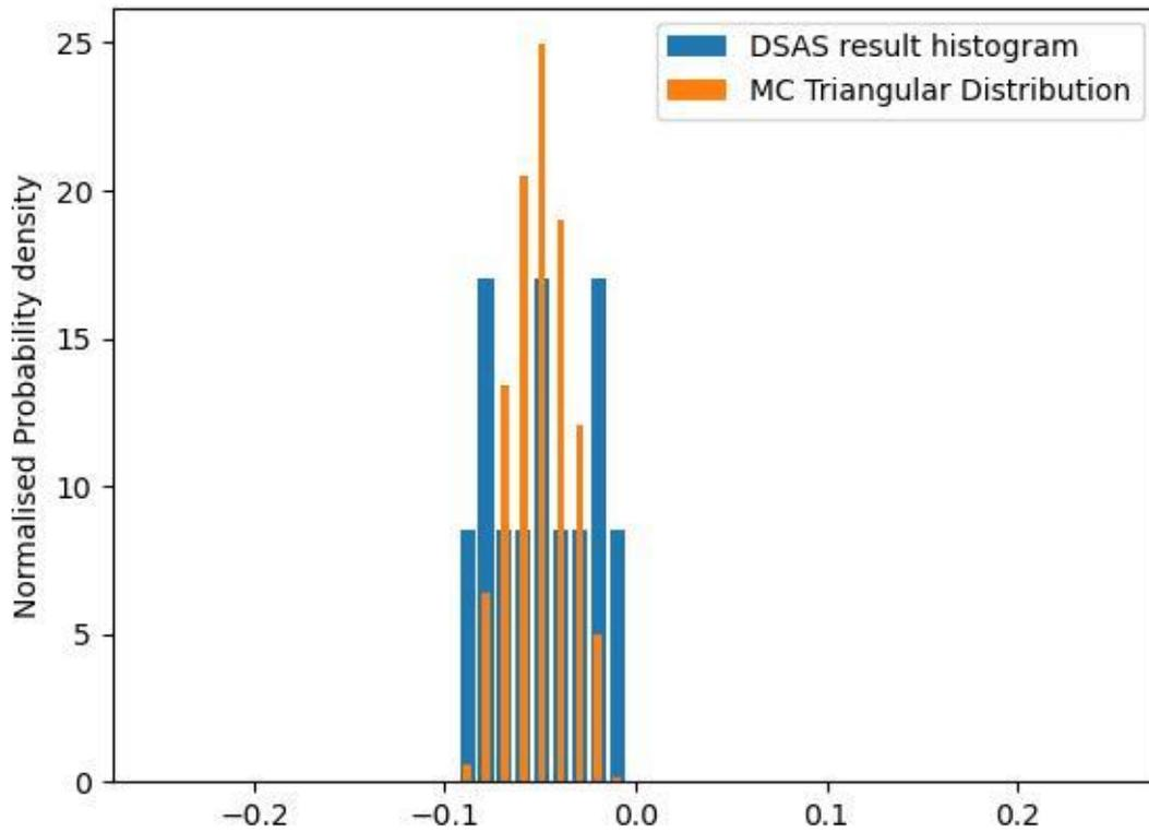
Figure 3-4 Shoreline Change Results for TCSC 41 (Frankston Pier) (positive is erosion)
