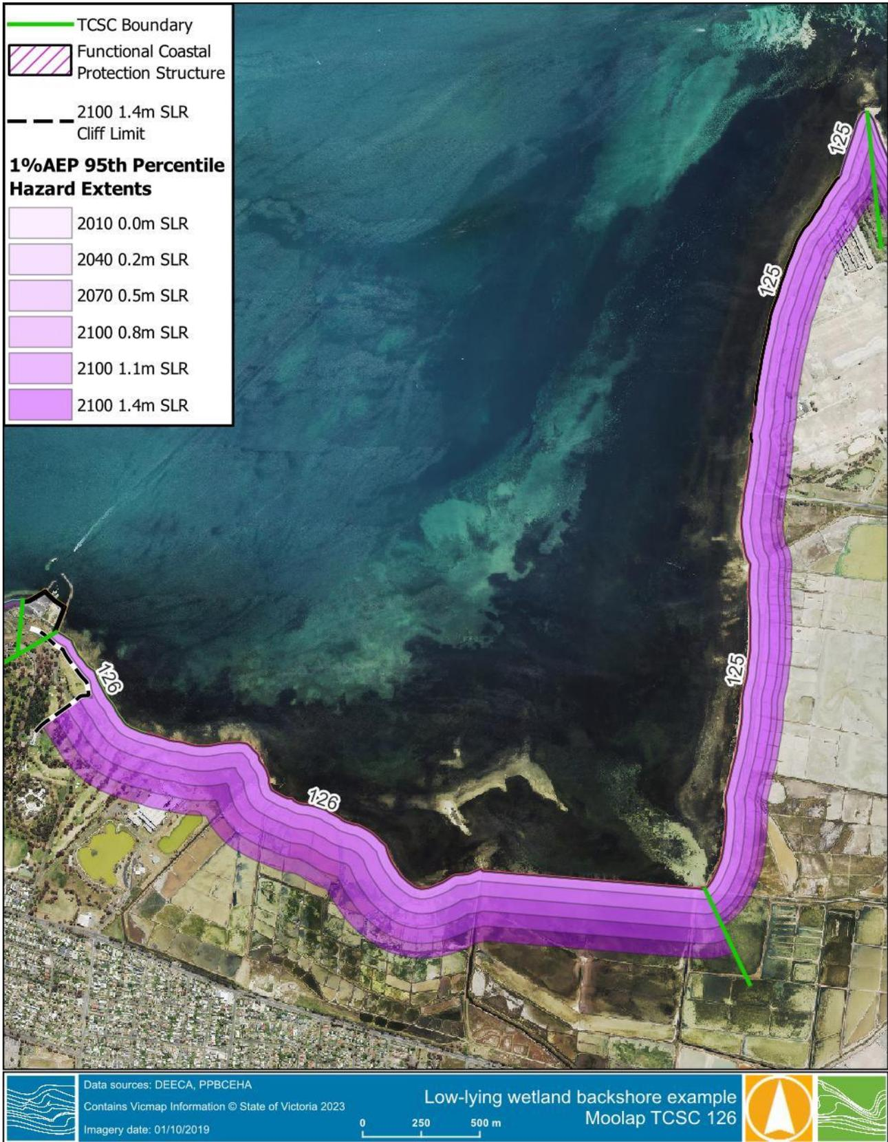
Figure 5-9 Backshore Wetlands Example from 95<sup>th</sup> Percentile 1% AEP
