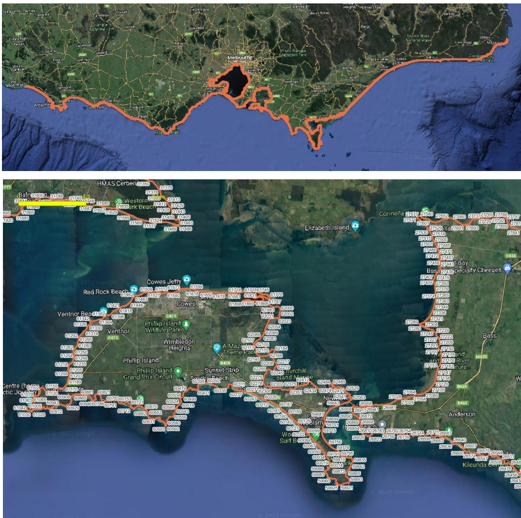
Figure 1.1. Victorian Coastal OmniLine transect framework, (top) full extent, (bottom) zoom in around Phillip Island, showing universal identifiers (UID).
