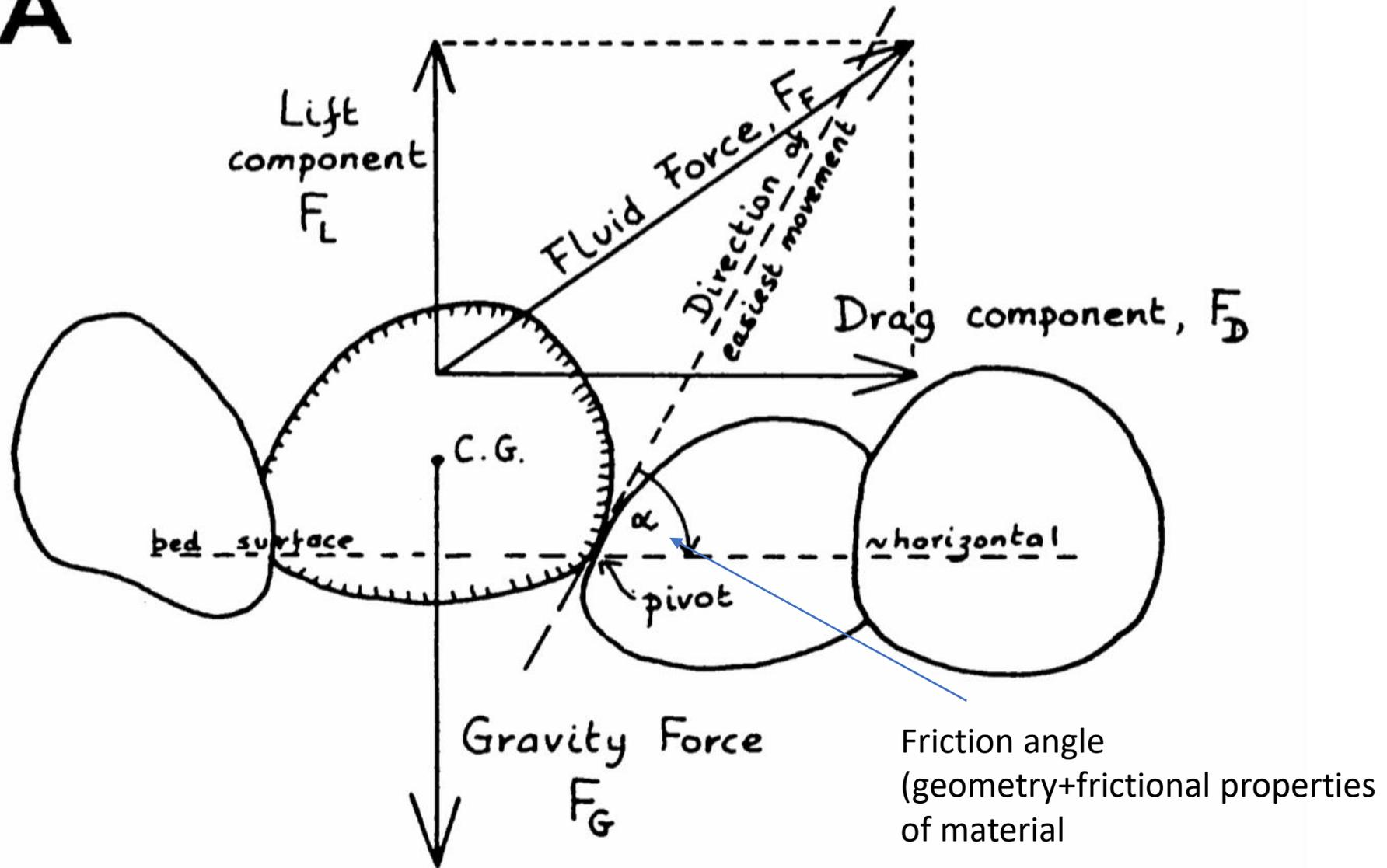
A range of moments operate on a sand particle: fluid force, gravitational force, drag
